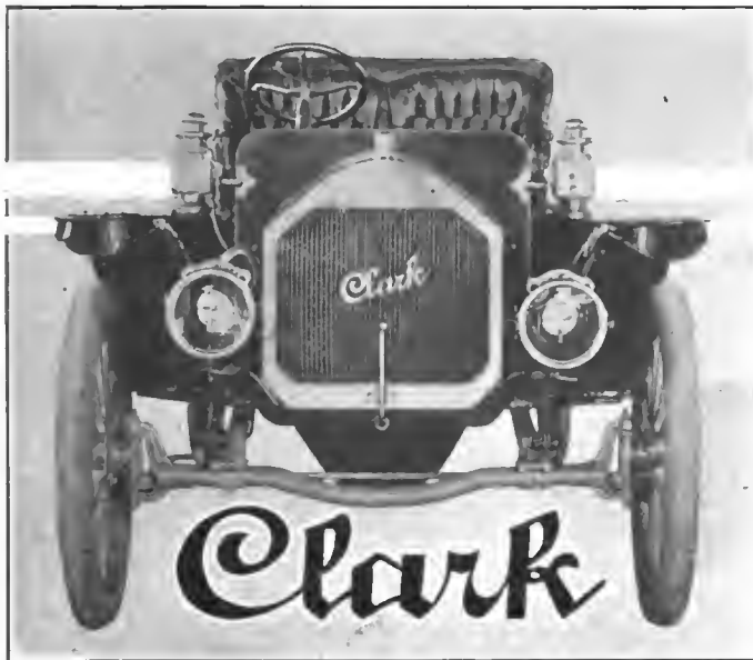
Showing Tubular Axle with Connections Well Protected
